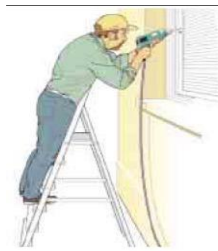
Correct – steps facing work activity
