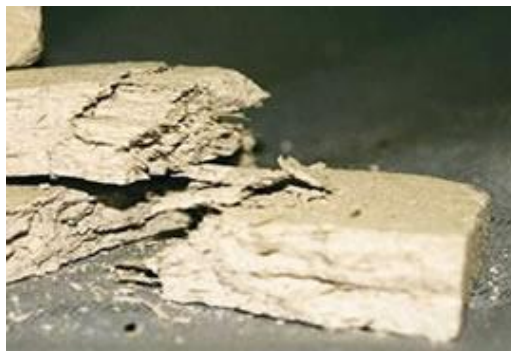
Pieces of Asbestos Insulating Board (AIB)
