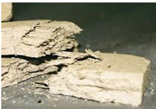
Pieces of Asbestos Insulating Board (AIB)
